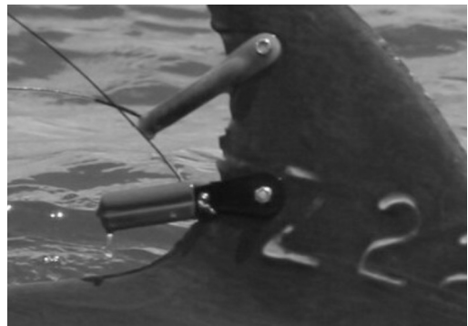
Figure 5b. Day 20: Z22 with no migration and no biofouling of satellite-linked transmitter
